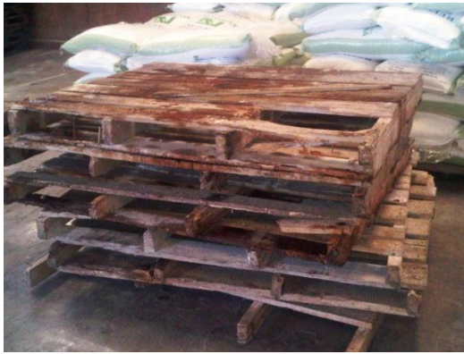
Figure 3. Faulty pallets in use
